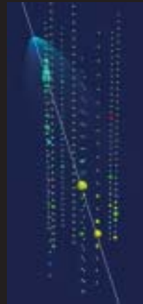
The IceCube telescope and its predecessor, AMANDA, use optical sensors to locate the sources of high-energy neutrinos. This picture shows the on-line display of a neutrino event recorded by AMANDA.
